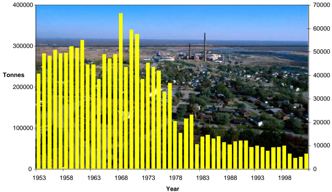
**Figure 2-30 Falconbridge Limited Sudbury Operations Sulphur Dioxide Emissions**
